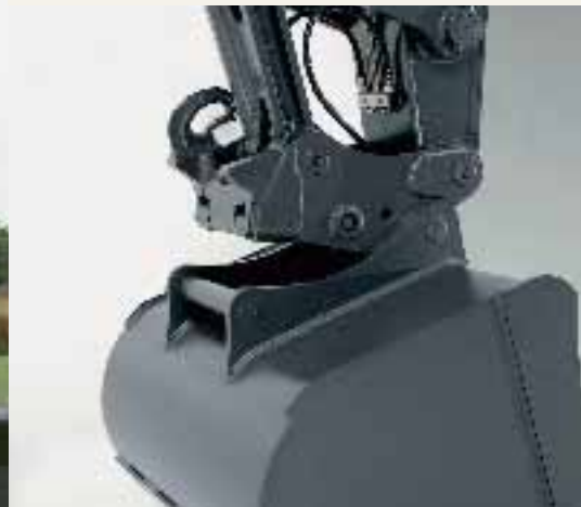
• Quick fit: easily change tools from the cab.
