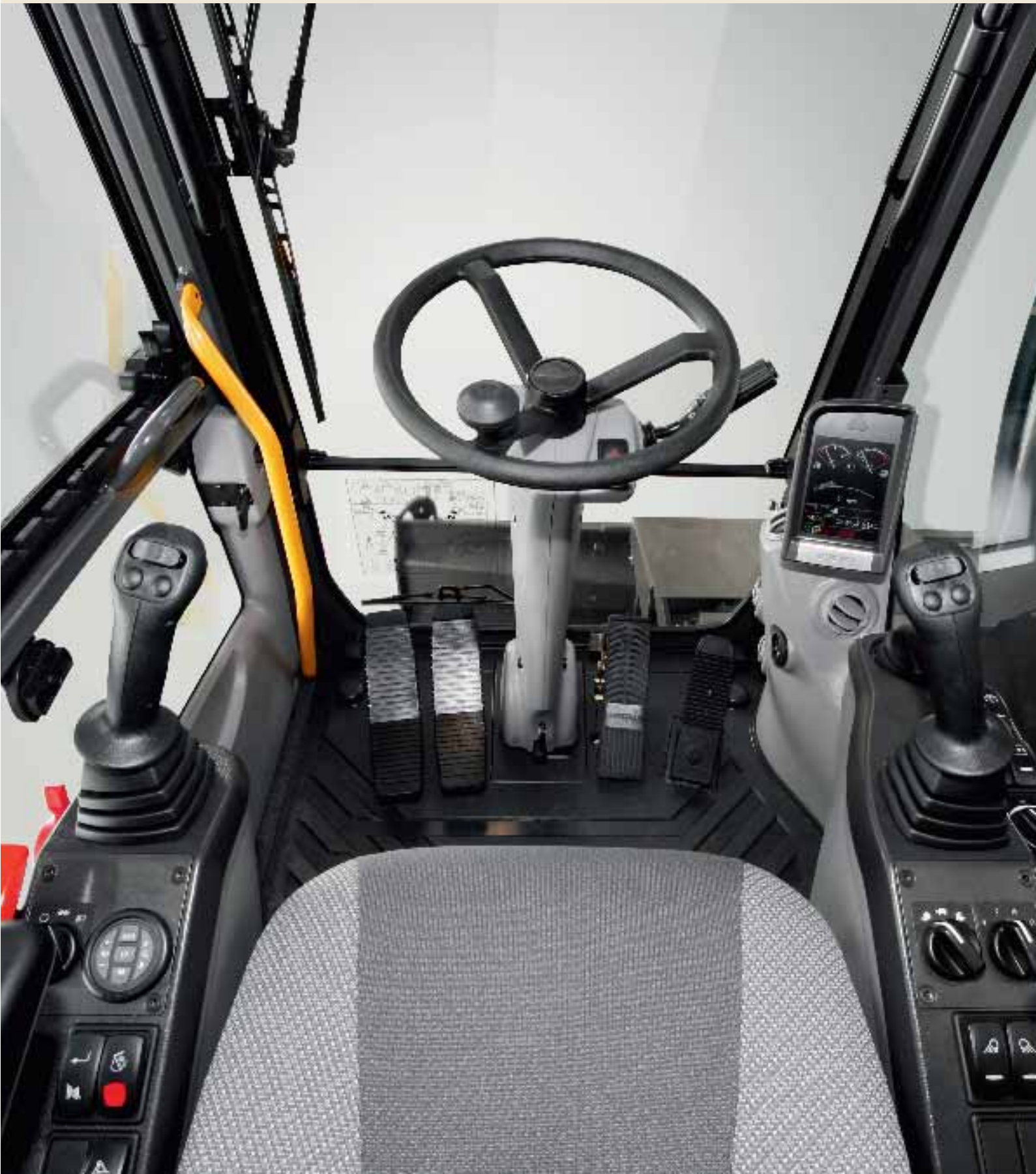
• Steering column pivots for visibility and comfort.
