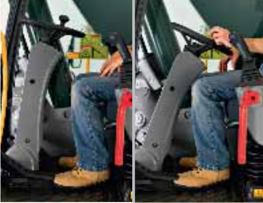
• Steering column pivots for visibility and comfort.
