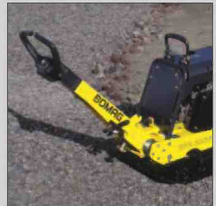
Steering rod with height-adjustment and locking device
