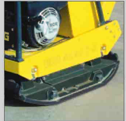
High wear resistant self-cleaning GGG 60 base plate. Depending on model and type working widths are available from 450mm up to 820 mm.
